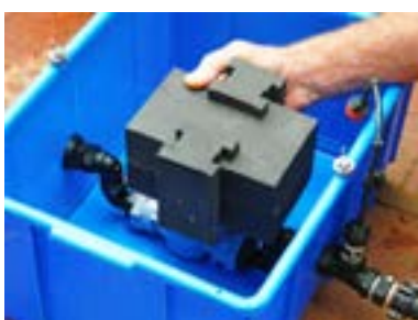
Position the float over the solenoid
