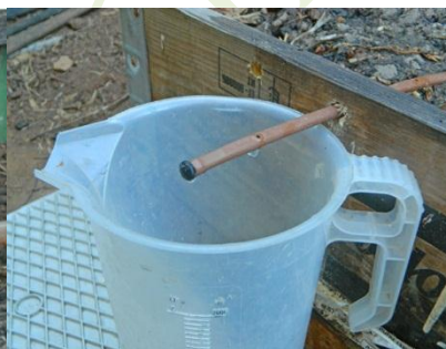
Remove water from the evaporator until the irrigation starts
