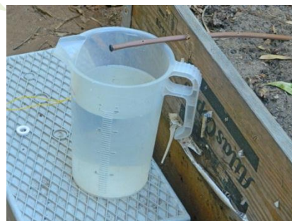
Dripper control volume in the measuring container
