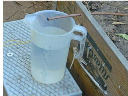
Dripper control volume in the measuring container
