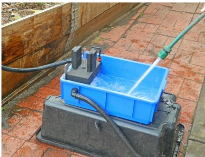
Fill the evaporator with water until the water level reaches the high level
