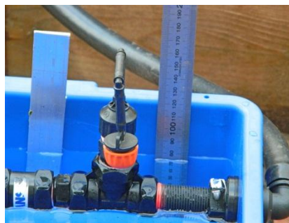
Measure the depth of water in the evaporator at the low level
