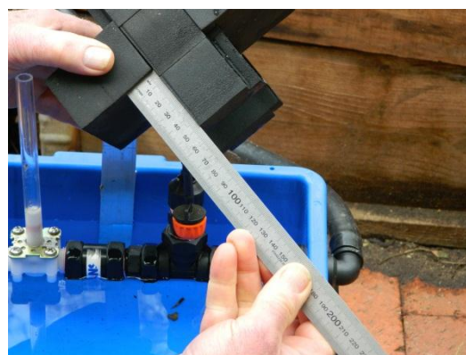
50 mm gap between the bottom of the float and the bottom of the slides
