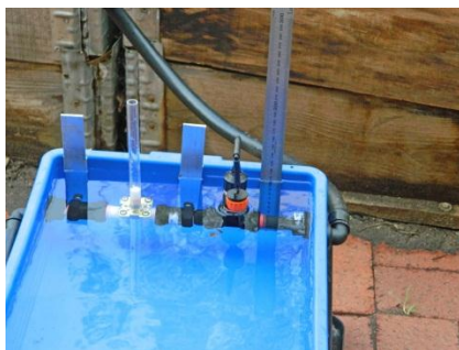
While the soil is drying, the water level in the evaporator is falling due to evaporation
