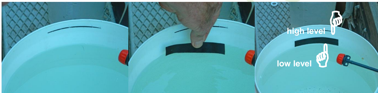
While the soil is drying, the water level in the evaporator is falling due to evaporation
