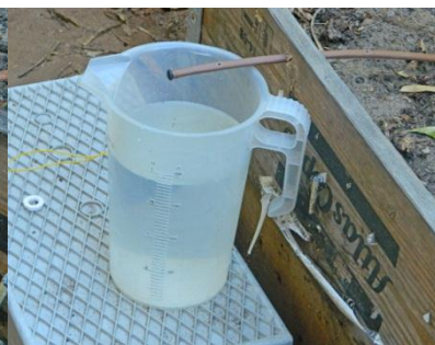
The irrigation stops automatically when the water level reaches the high level
